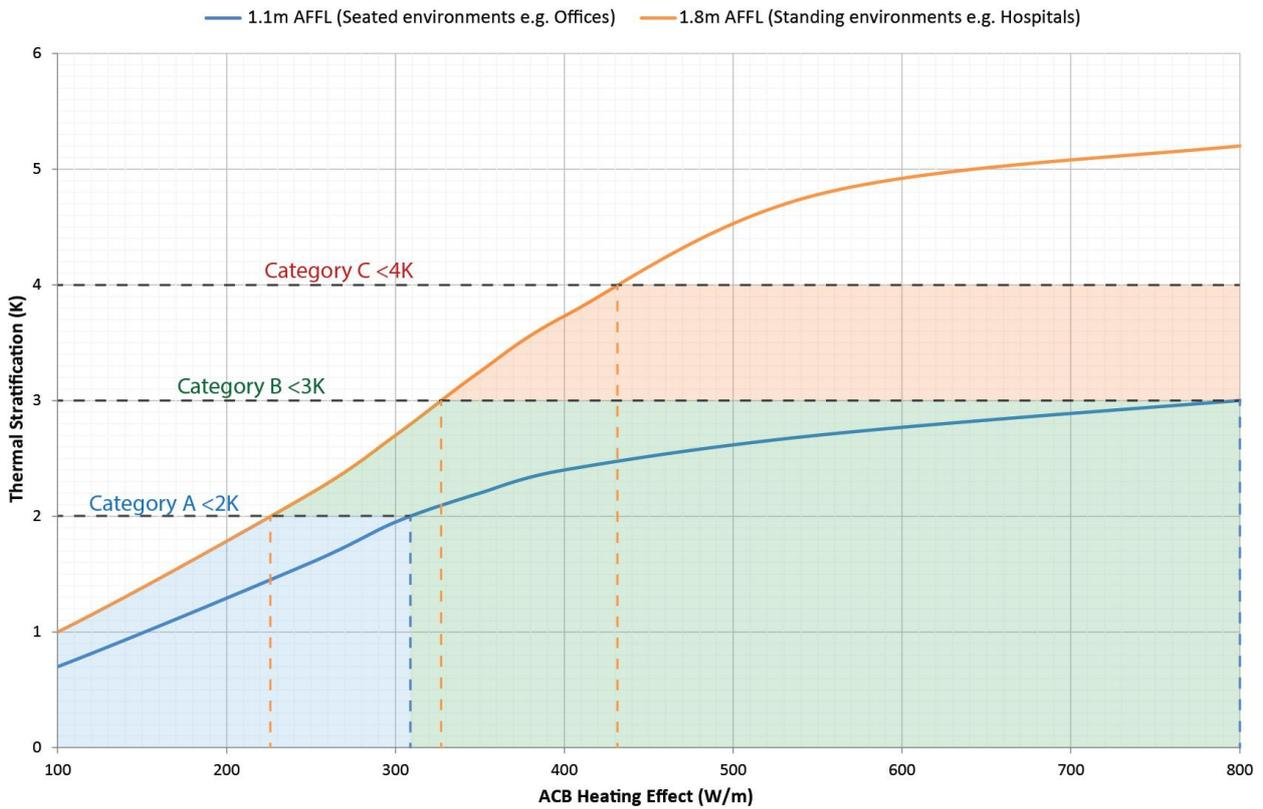
Note: The above relationships have been based on extensive Compact and Eco active chilled beam heating tests based on a worst case scenario i.e. Full height low surface temperature glazing and steady state conditions with no mixing of room air which simulates an unoccupied building.
