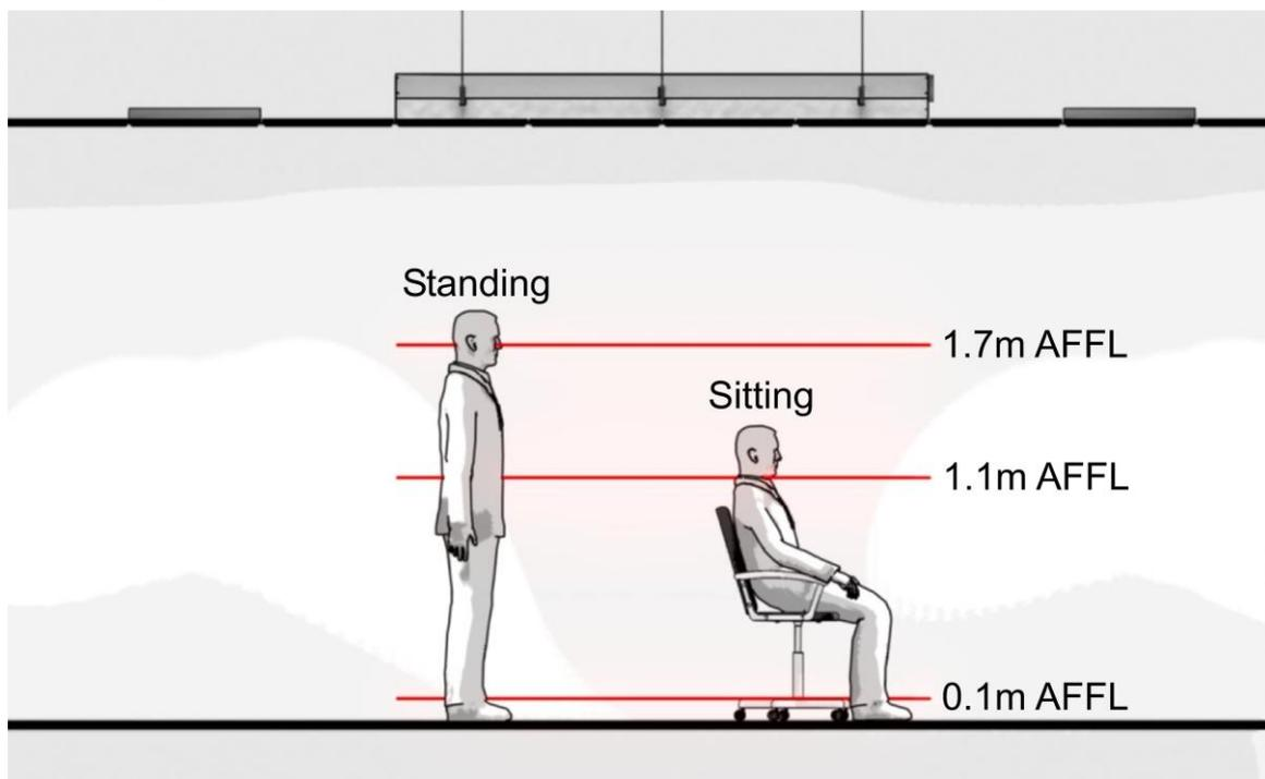
The following chart can be used to determine anticipated levels of thermal stratification within the occupied zone:
