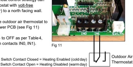
**WARNING:** Do not apply any voltage to terminal IN1 as this will damage the Ecopower PCB.
