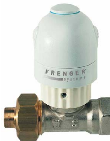
The actuator mounted on the valve. Actuators (NC) and valves with valve function are usually supplied closed in a non-current mode. The pipe fittings shown in the picture can be ordered separately.
